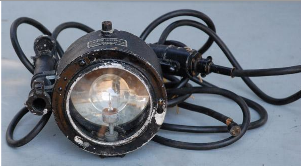
Above and below: 4 inch Aldis lantern, pattern S5110E. Made by Sutton-Horsley Co. Ltd, of Toronto Ontario. This one was last used on HMCS Labrador. Since there was no battery compartment in the carrying case and the lamp has a long power cord, it is believed it was powered from the ship's low voltage power mains. Five inch Aldis lamps produce 150,000 candlepower. (Photo by Jerry Proc)
