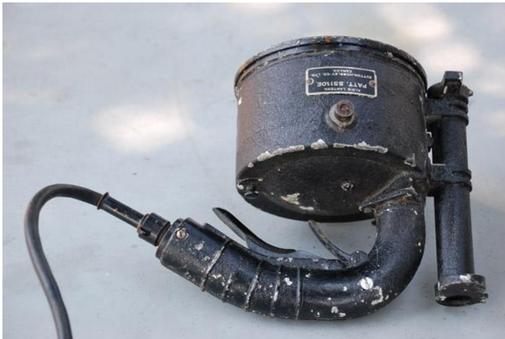
Above and below: 4 inch Aldis lantern, pattern S5110E. Made by Sutton-Horsley Co. Ltd, of Toronto Ontario. This one was last used on HMCS Labrador. Since there was no battery compartment in the carrying case and the lamp has a long power cord, it is believed it was powered from the ship's low voltage power mains. Five inch Aldis lamps produce 150,000 candlepower. (Photo by Jerry Proc)
