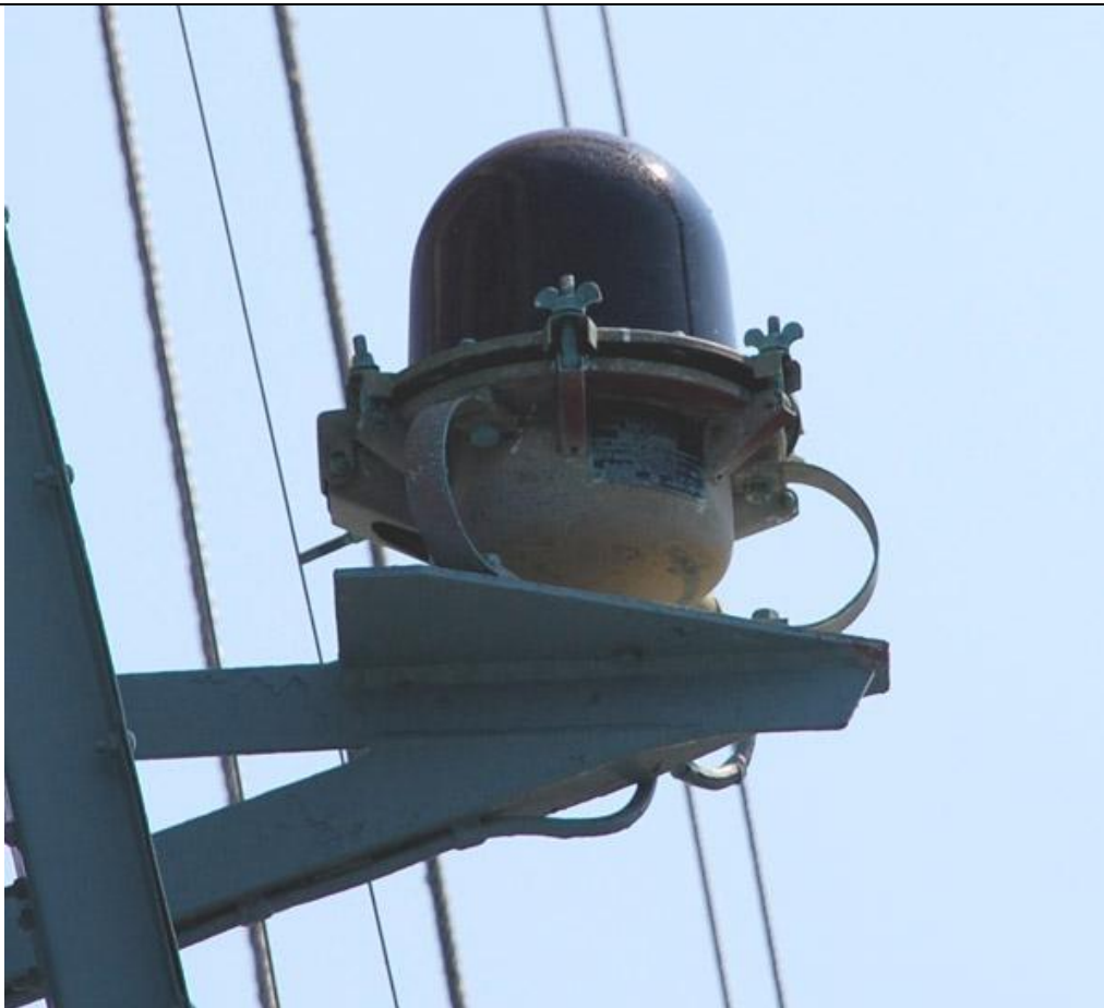
Close-up of an infrared lamp. Keith Kennedy also confirms that infrared signalling was referred to as "Nancy" in the RCN. Sometimes a reddish coloured infrared filter would be placed over the 10 inch signal projector for infrared signalling but it resulted in a reduction in the size of the beam. Infrared signalling was sometimes referred to as "dark light" signalling. ( Photo by Jerry Proc )
