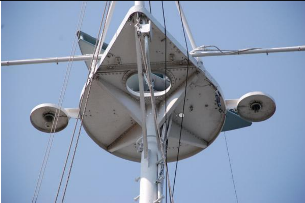
Close-up of the flashing masthead lights attached to the 293 platform. The truck lights atop the shade cannot be seen from this angle. (Photo by Jerry Proc)
