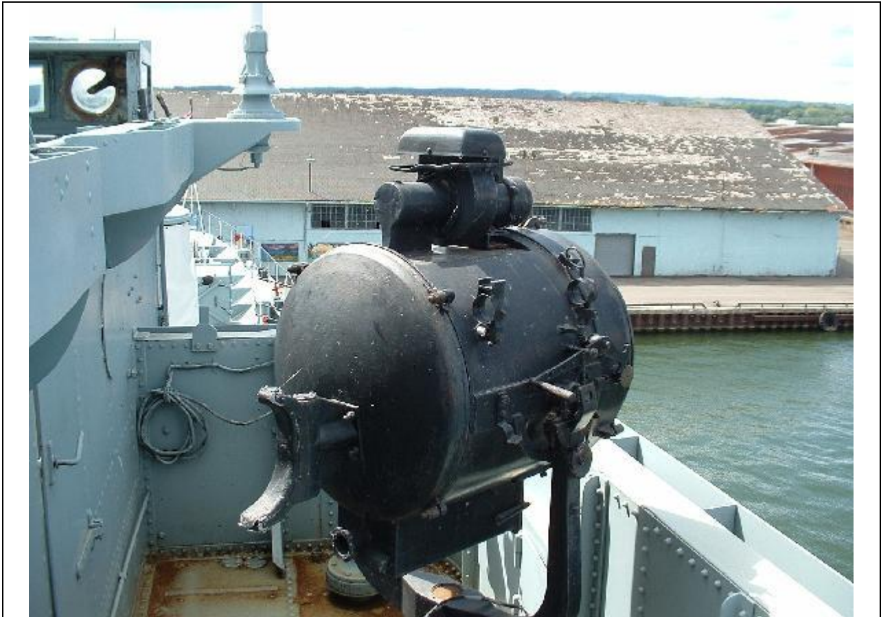
Starboard side 20 inch signal projector aboard HMCS HAIDA Type 170A Mk IV. It could also double as a searchlight. (Photo by Jerry Proc)
