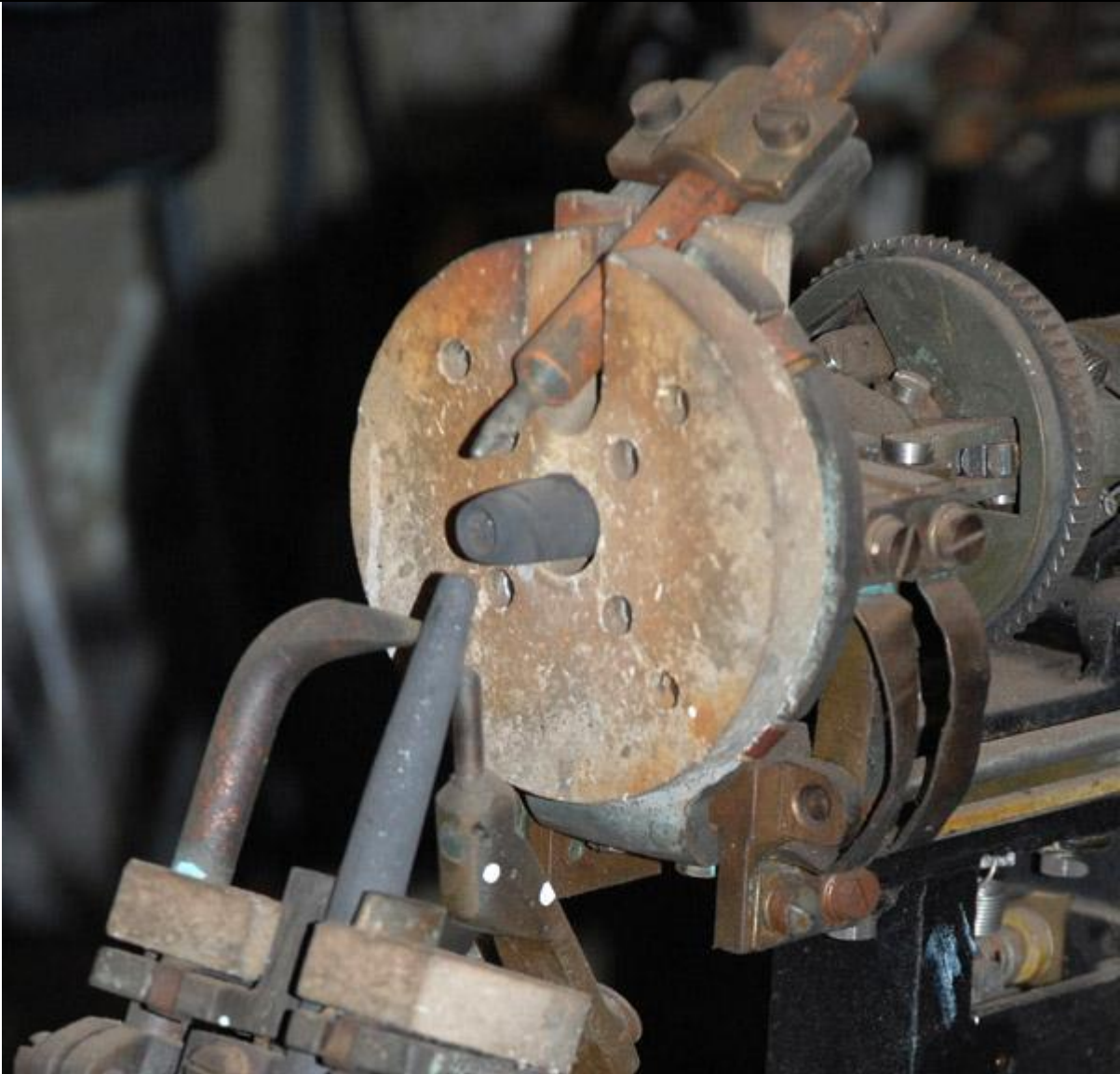
Closeup of the carbon arc elements which consume 5700 watts of power in this model. After the arc is flashed up, an internal motor rotates the carbon rods slowly and at the same time a ratchet mechanism pushes them forward to maintain a constant gap as the heat consumes the carbon. Without a drive mechanism for the carbon rods, it would be an impossibility for a signalman to keep the arc lit, train and elevate the light and operate the shutters while a ship was rolling and pitching! (Photo by Jerry Proc)
