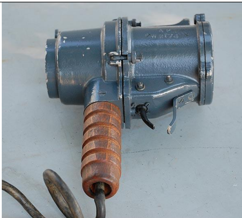
Intermediate Lantern - Side view. Admiralty Pattern Number AP2174. ( Photo by Jerry Proc )
