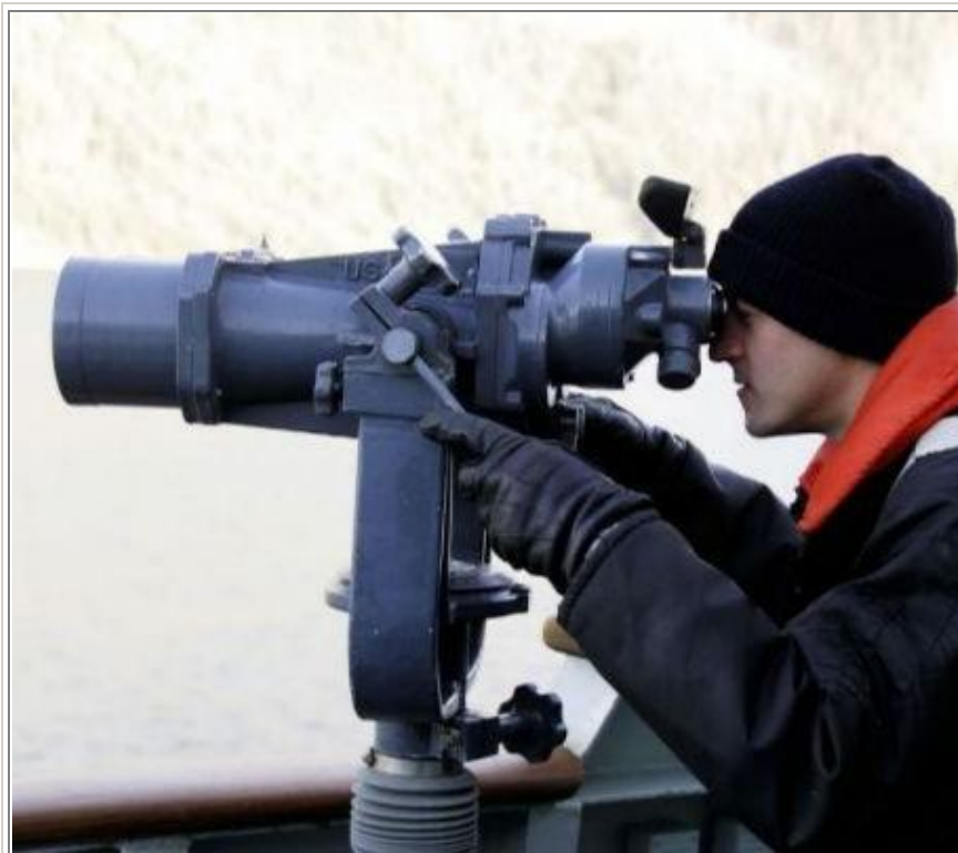
Big Eye in action. The binocular assembly weights 22.7 Kg; carriage assembly is 39.5 Kg; Pedestal assembly is 26.3 Kg. (DND photo)
