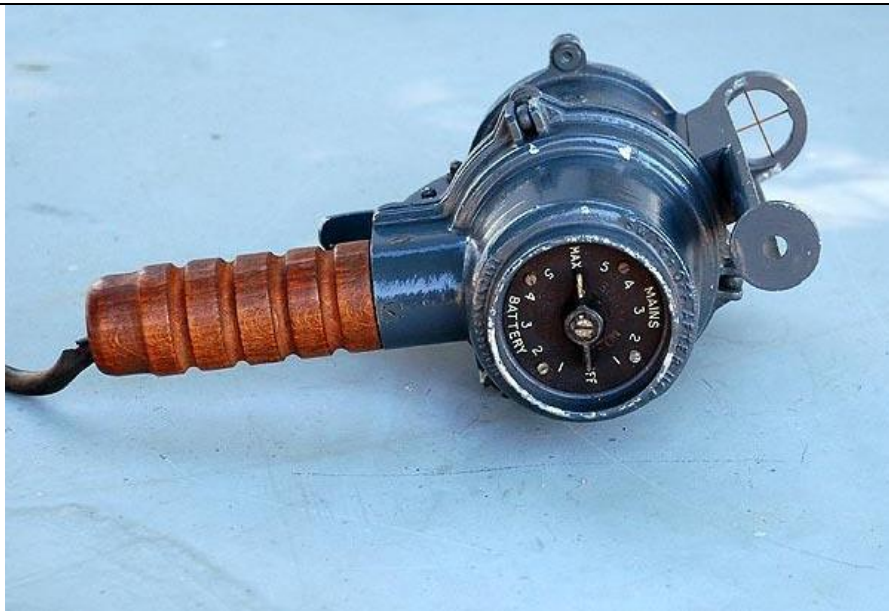
Intermediate Lantern - Rear View. The control dial selected the power source (mains or battery) and the light intensity for each power source. (Photo by Jerry Proc)
