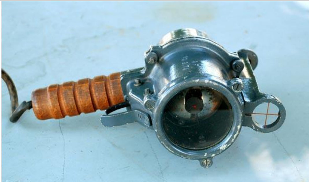
Intermediate Lantern - Front view. The black cylindrical object in front of the mirror is the shutter. It moves forward when the trigger is engaged thus allowing light to escape. ( Photo by Jerry Proc )
