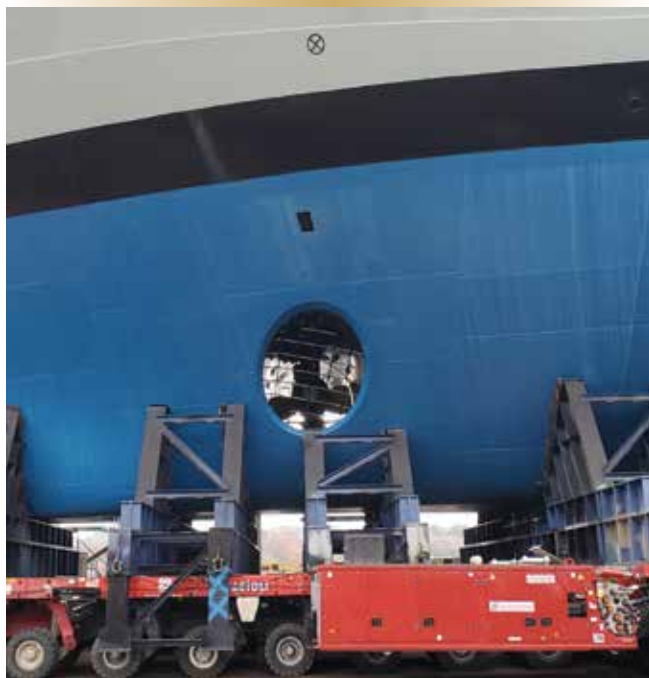
Figure 5. The AOPV transverse tunnel bow thruster.
