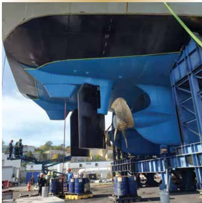
Figure 4. The AOPV rudders are well protected for operation in ice.
