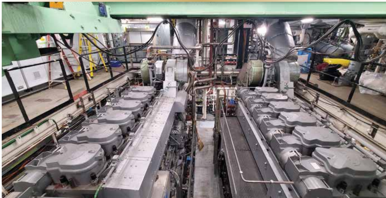
Figure 1. Two of the AOPV's four 3600-kW MAN diesel engines that provide electrical power for propulsion and ship electrical systems.
