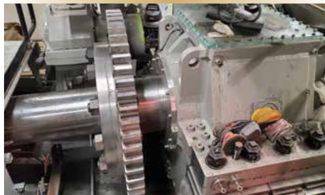
Figure 2. Thrust block and turning gear arrangement.
