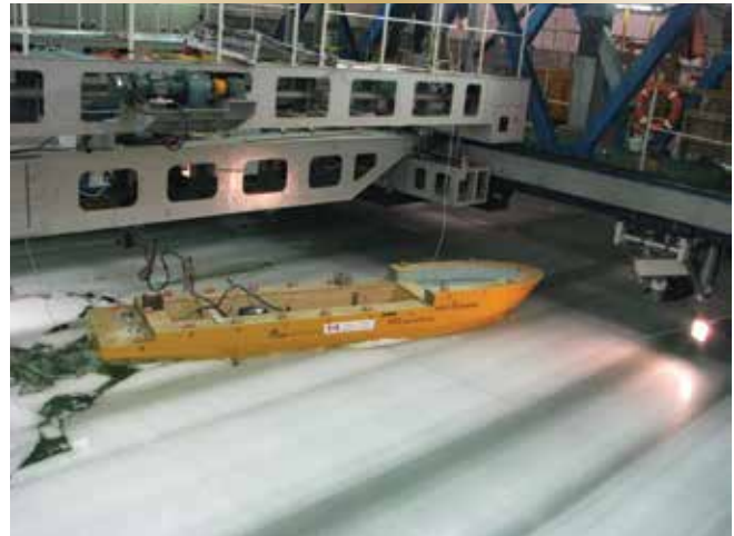
Figure 3. AOPV tank testing in ice at the National Research Council's facility in St. John's, NL.
