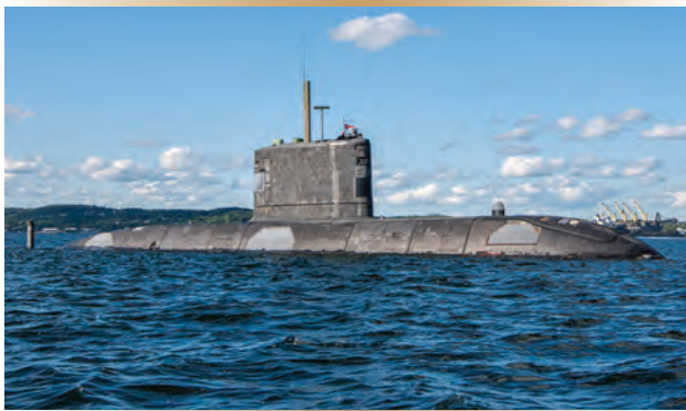
Figure 1. Victoria -class (ex- Upholder ) submarine pressure hulls were built to UK MoD engineering standards, based on UK Defence Science and Engineering knowledge and experience.
