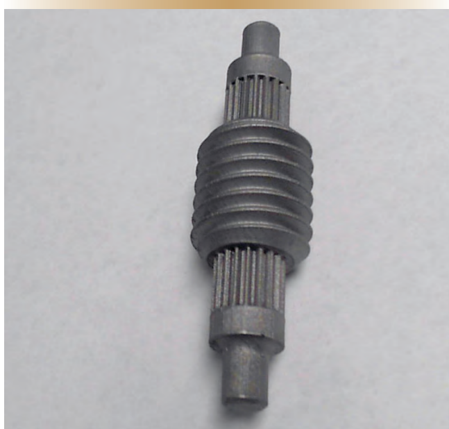
Figure 3. Metal – 316L stainless steel worm gear.
