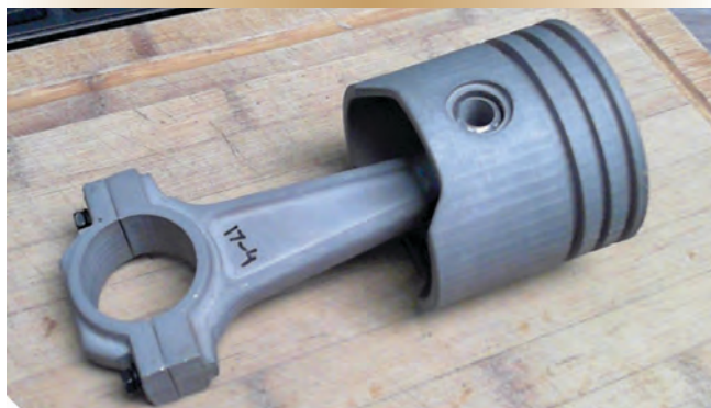
Figure 2. Metal AM proof-of-concept items include this 17-4 stainless steel piston (left), and a compound impeller manufactured in copper.
