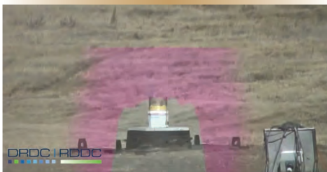
Figures 4a and 4b. The moments of detonation. The pink area is a video capture of the beginning of the shock wave.
