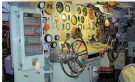
Figure 1. The steam throttles and other machinery controls and gauges on the engine-room console of a Restigouche -class destroyer escort.
