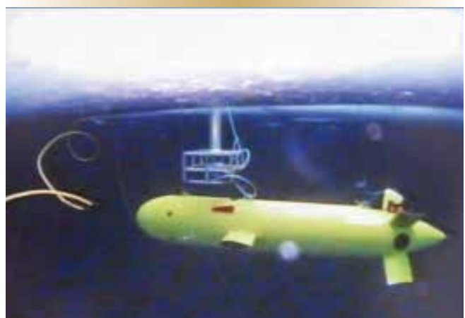
Figure 1. AUVs working under ice or at great depth rely on inertial systems for navigation, but do not have access to GPS information to correct for small INS drift errors.
