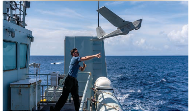
Figure 2. A Puma RPAS being hand-launched from a Kingston -class MCDV.
