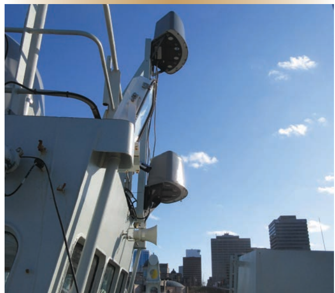
Figure 4. The MCDV superstructure antenna arrangement for the Puma RPAS went through several iterations of development, design and integration to achieve a best fit.
