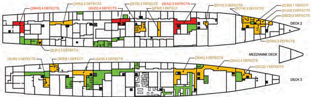
Figure 8. An example of a deck survey heat map showing the frequency and location of defects.
