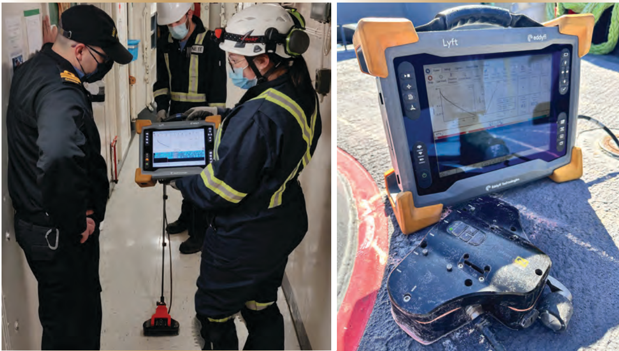
Figure 3. PEC shipboard scanning trials with the custom 7-channel eddy current probe.
