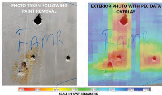
Figure 6. Examples of known defects and corresponding scan results from a 2022 hull survey.
