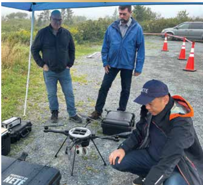
NETE personnel prepare a Teledyne FLIR SkyRanger R70 UAV for a test flight.
